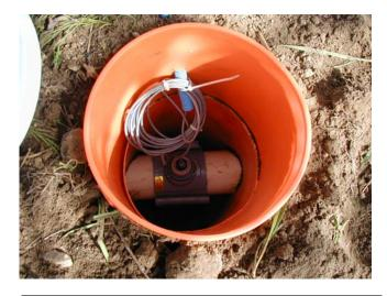
Meter installed in saddle in "bucket" vault.
